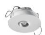
Extension movement detector white, recessed. To be used when the area to be covered is bigger than 6,00x5,00m by height 2,50m. To be connected to one of the outputs of the INTERACTIVE-DALI controller. No extra mains connection required. M074130
